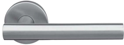
106 Square Profile: V2 Spindle 8mm Base Material: Stainless Steel AISI 304. Guide: 16 mm in Brass. Finish: SSS, PSS
