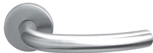
108 Square Profile: V2 Spindle 8mm Base Material: Stainless Steel AISI 304. Guide: 16 mm in Brass. Finish: SSS, PSS
