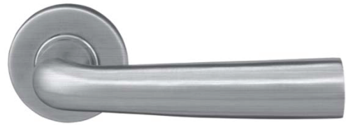
156 Square Profile: V2 Spindle 8mm Base Material: Stainless Steel AISI 304. Guide: 16 mm in Brass. Finish: SSS, PSS
