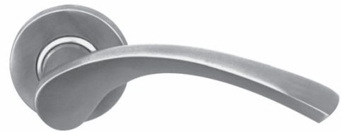
154 Square Profile: V2 Spindle 8mm Base Material: Stainless Steel AISI 304. Guide: 16 mm in Brass. Finish: SSS, PSS
