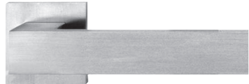
146 Square Profile: V2 Spindle 8mm Base Material: Stainless Steel AISI 304. Guide: 16 mm in Brass. Finish: SSS, PSS
