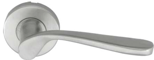
166 Square Profile: V2 Spindle 8mm Base Material: Stainless Steel AISI 304. Guide: 16 mm in Brass. Finish: SSS, PSS
