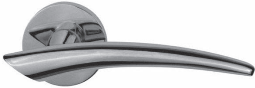
163 Square Profile: V2 Spindle 8mm Base Material: Stainless Steel AISI 304. Guide: 16 mm in Brass. Finish: SSS, PSS
