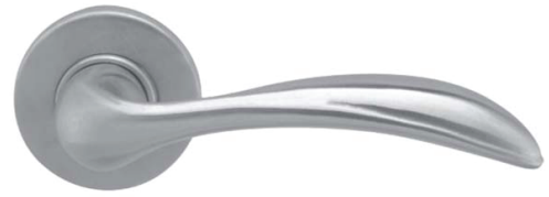
132 Square Profile: V2 Spindle 8mm Base Material: Stainless Steel AISI 304. Guide: 16 mm in Brass. Finish: SSS, PSS
