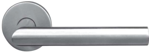
109 Square Profile: V2 Spindle 8mm Base Material: Stainless Steel AISI 304. Guide: 16 mm in Brass. Finish: SSS, PSS
